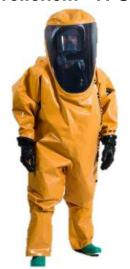
The Trellchem VPS-Flash material combines a flame retardant aramid base fabric with abrasion resistant rubber and a multilayer chemical barrier film. All together it provides over 8 hours permeation time against a wide variety of hazardous chemicals along with flash fire protection and protection against liquefied gases, radioactive particles and biohazards
