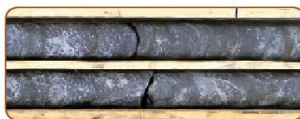
Example of Magnetite in Veins from Mariposa Total iron grade: 60% max, 30% average
