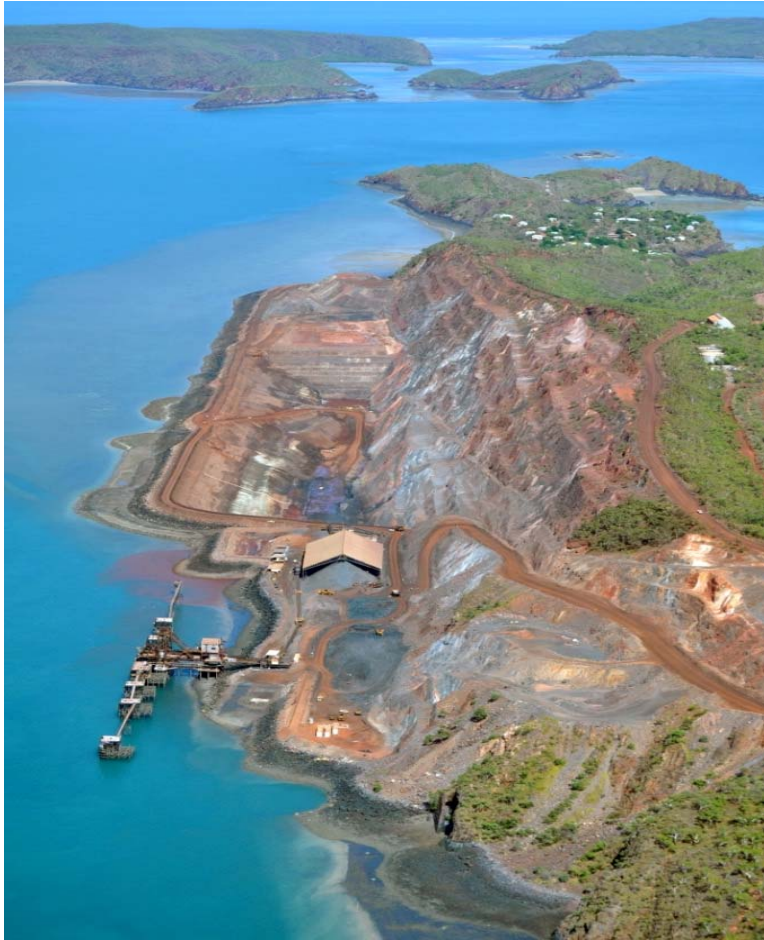
Photo of Cockatoo seawall operations with stockpile shed and crusher sitting above Stage 4 ore body. Irvine Island top left.
