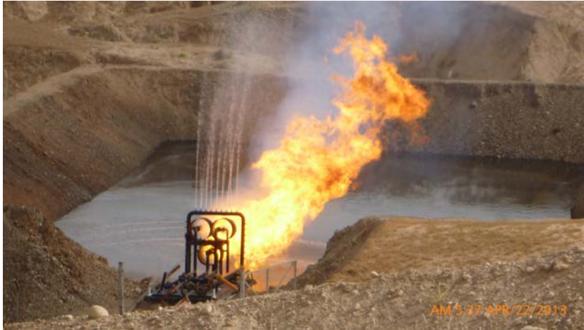
Open hole test of lower zone of Taza 1 well, Kurdistan.
