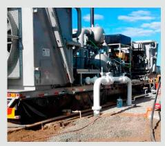
The new 1,000 HP trailer-mounted booster compressor – believed to be the first unit of its type in Queensland.
