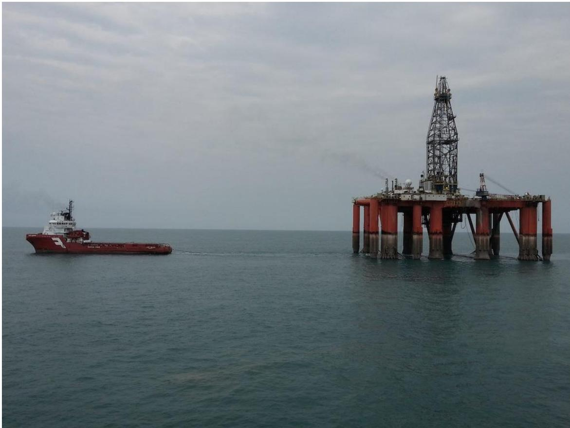
Image of semi-submersible drill rig Stena-Clyde under tow
